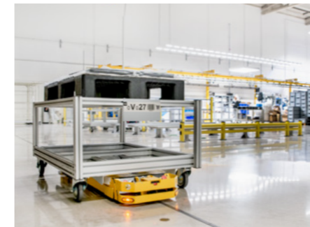
Automated guided vehicle for flexible internal logistics
