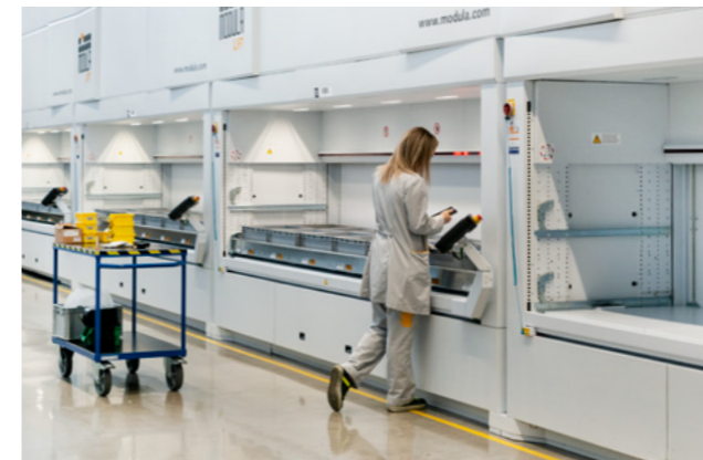
Automated vertical storage system
